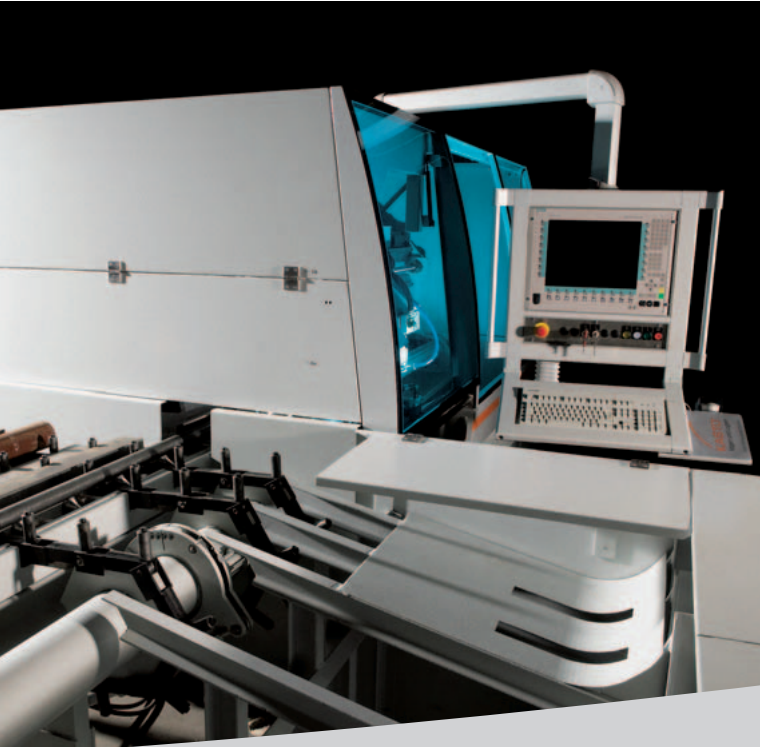
KASTO TechnoControl : Easy shop-oriented operation with menu control via function keys.
