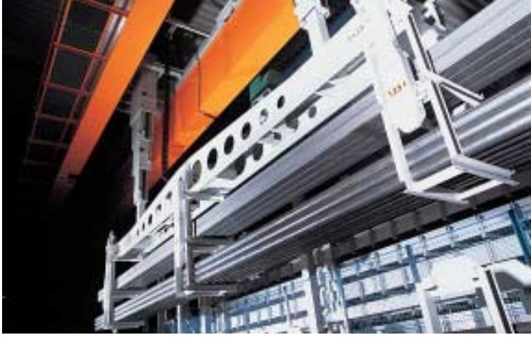
Fast transport: Multiple lift spreader beam with three adaptor pairs and telescopic guide while moving 2 storage layers
