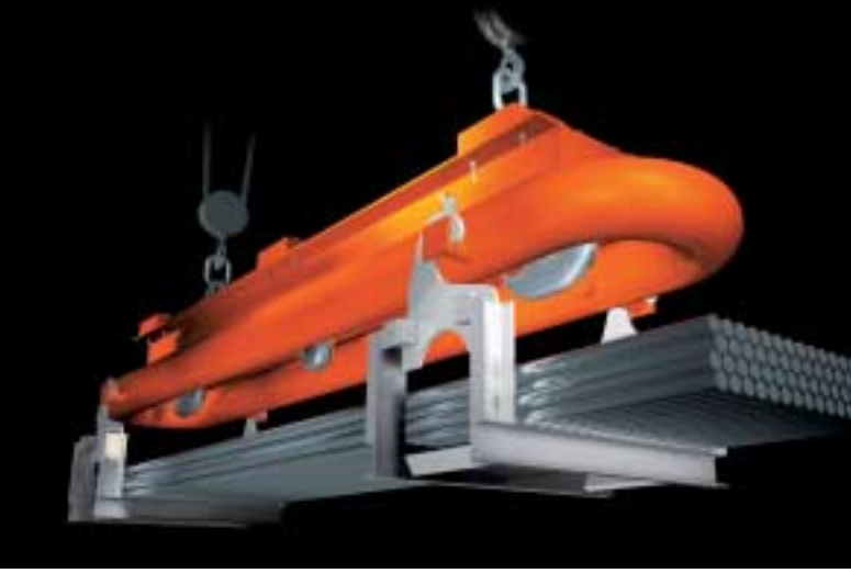
UNIBLOC E : The starter version regarding stacking cradles : Moving a KASTO-cradle type UNIVERSAL
