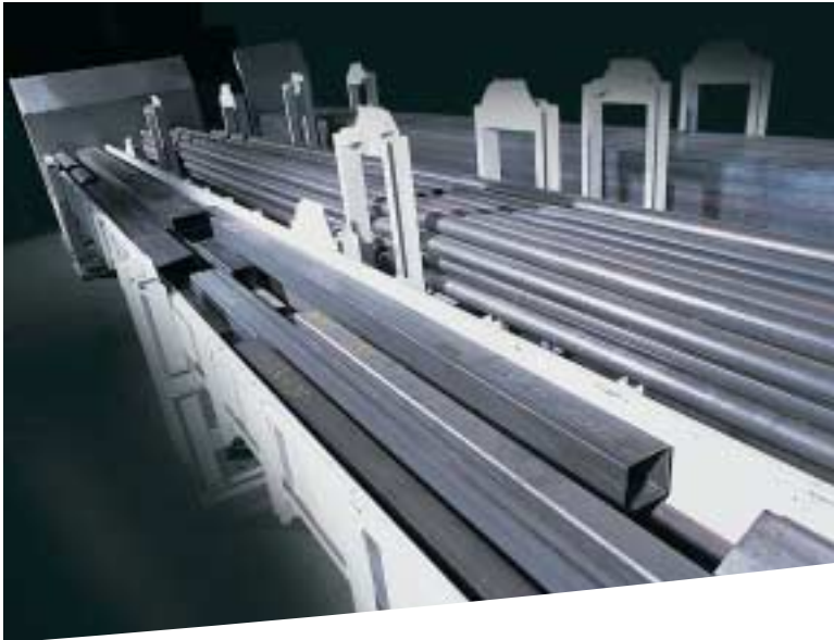
Flexible storage: Even remnants can be optimally stored by using stacking cradle cassettes
