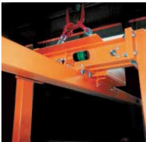
Optical display of gripper function for safe and fast cradle handling
