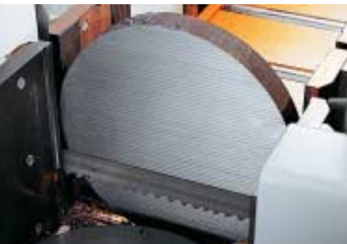
Less scrap, more profit: minimal rest piece length 35 mm in automatic operation.
