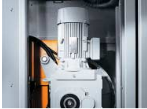
Strong and sensitive: frequency regulated helical-bevel motor directly at the drive wheel with concentric bearings.
