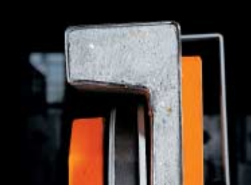
Mechanical engineering up-to-date: steel casing of KASTOtec's saw head filled with polymer casting.
