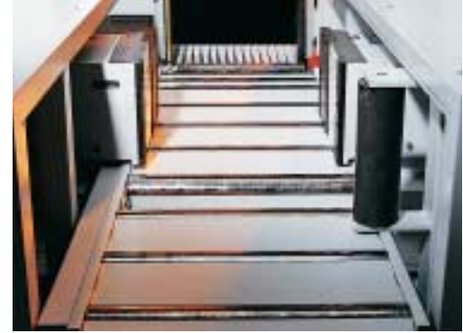
The continuous integrated machine roller conveyor simplifies material handling and transportation of short remnants.
