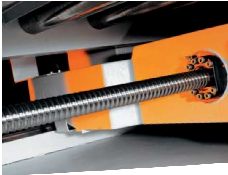
Highly accurate and durable feed with recirculating ball screw with little maintenance.
