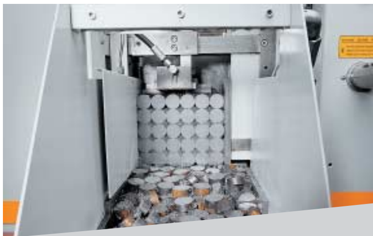
Motor-driven vibrating table with cleaning unit for virtually chip-free cuts (optional).
