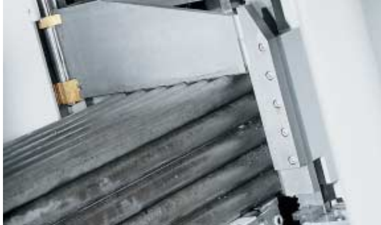
Hydraulic hold-down device for stable 4-point clamping of individual bars, material layers and bundles (optional).
