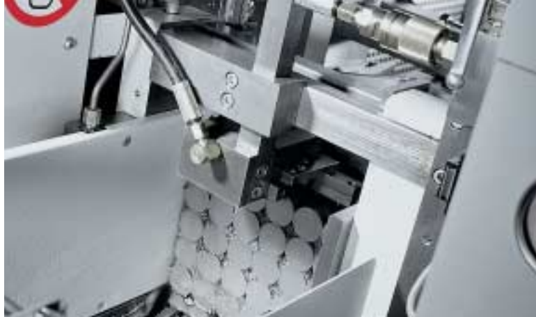
For bundle cuts: The „top-down“ hydraulic clamping device (optional).
