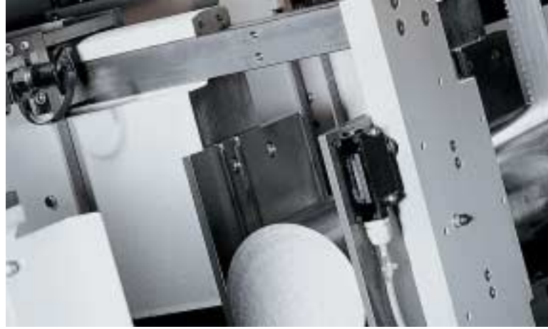
The frame clamping vice prevents the material from moving up.
