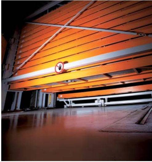
Lateral station - carriage, can be moved out on both sides
