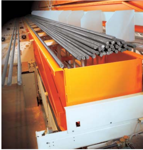
Lateral station – chain conveyor with push-up device
