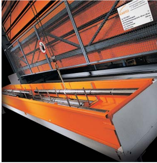
Lateral station - cassette conveyor
