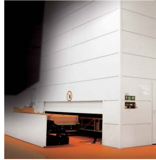
UNITOWER with cladding to protect the material
