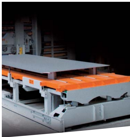
Longitudinal station - carriage with lifting device
