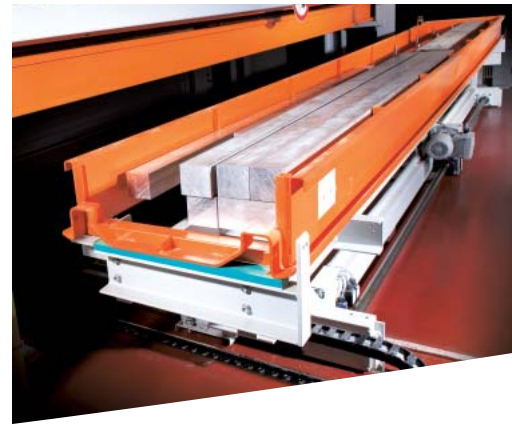
Lateral Station - carriage with a cassette open at front
