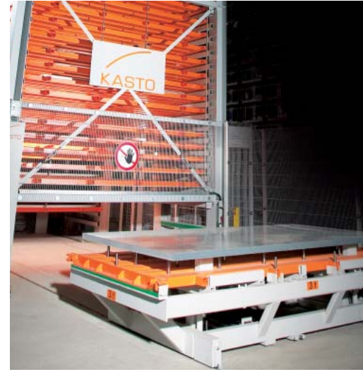
Lateral station - carriage with lifting device
