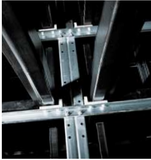
Durable and virtually wear free: Glide pads made of special plastic material.
