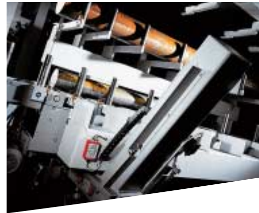
The KASTO quick-change station minimizes idle times when changing bars
