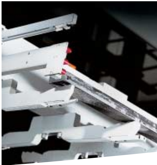
The specially designed KASTO loading traverse always removes and transports exactly one bar from the cantilever shelves.
