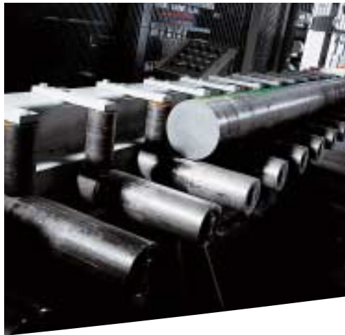
Outfeed roller conveyor to feed saws.
